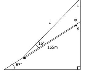
In order to find *L* using Law of Cosines, the height of the tower, and the angle between the tower and the hill need to be found.
