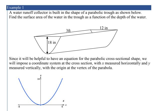
From this we find an equation for the parabolic shape. Since we placed the origin at the vertex of the parabola, we know the equation will have form  $y(x) = ax^2$ . Our equation will need to pass through the point (6,18), from which we can solve for the stretch factor *a*:
