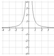
We get this behavior when the degree of the factor in the denominator is even. The distinguishing characteristic is that on both sides of the vertical asymptote the graph either increases or decreases.
