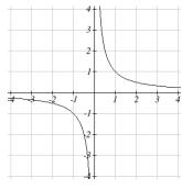
We get this behavior when the degree of the factor in the denominator is odd. The distinguishing characteristic is that on one side of the vertical asymptote the graph increases, and on the other side the graph decreases.
