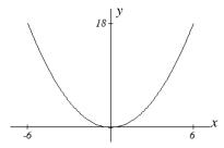
From this we find an equation for the parabolic shape. Since we placed the origin at the vertex of the parabola, we know the equation will have form  $y(x) = ax^2$ . Our equation will need to pass through the point (6,18), from which we can solve for the stretch factor a:
